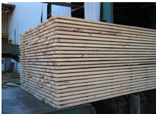
STACKING QUALITY improved airflow, minimized drying times and maximized quality, value & recovery.
