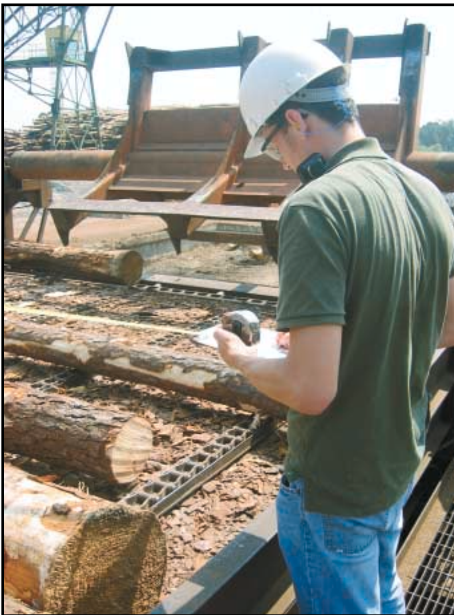
Quality control personnel conducts "logs on length" checks. This is one of the "controllables" that is used to gauge performance at the buck saw.
